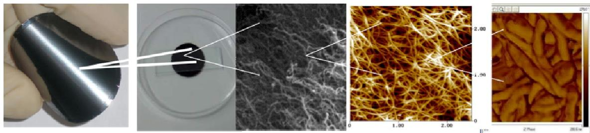
Figure 3: Processing of CNT into free-standing paper-like materials
